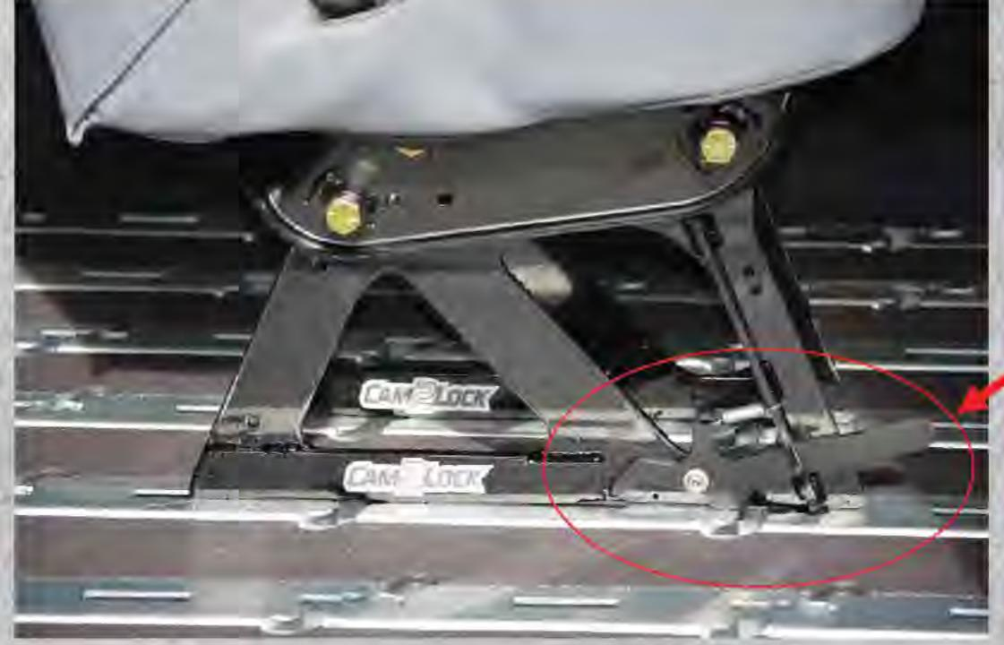
CAMLock2 allows Factory OEM Seat integration with an FMVSS seat base solutions
