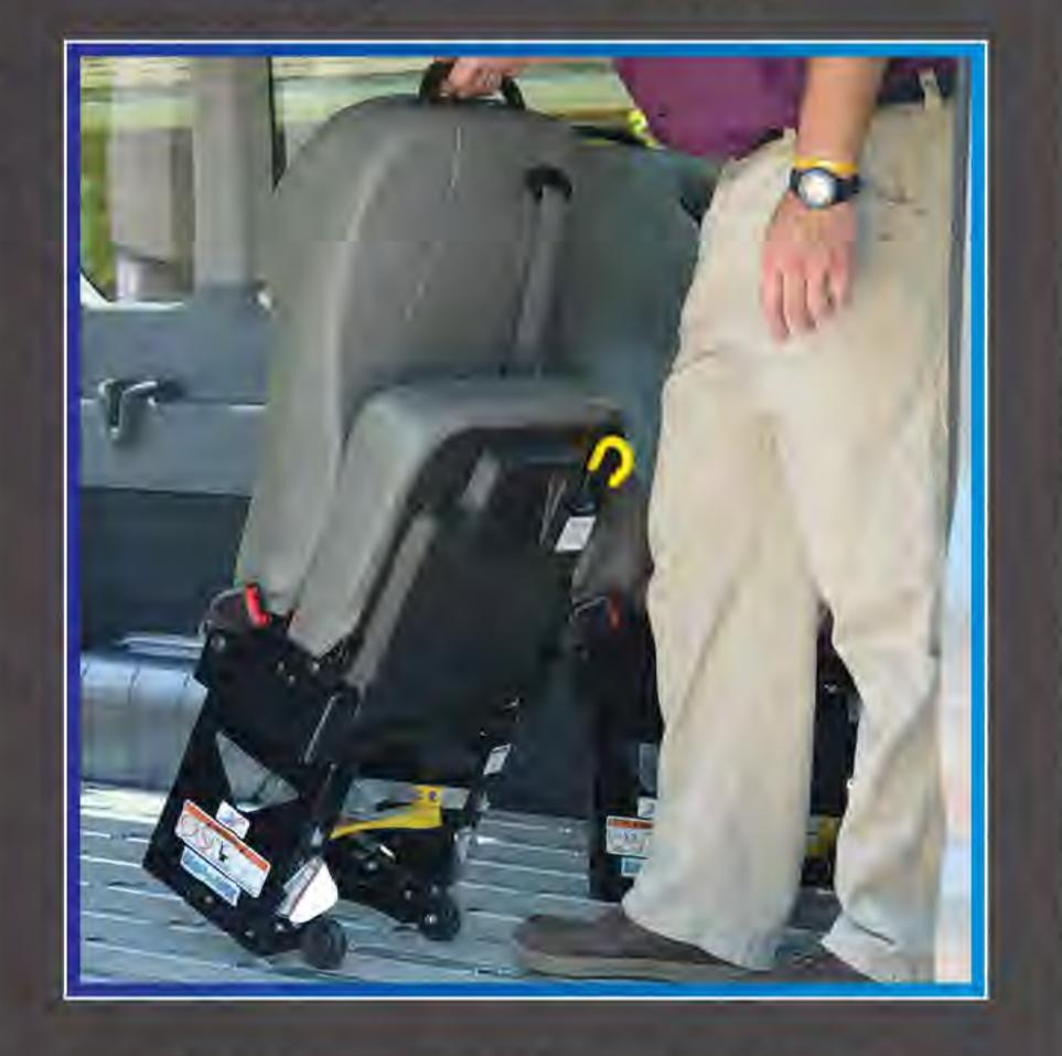
AbiliTrax provides drivers with a much more user friendly environment when they are changing seating configurations. By the driver simply using their foot, AbiliTrax allows for "hands free" latching and unlatching of the "Step N Lock" seat base.
