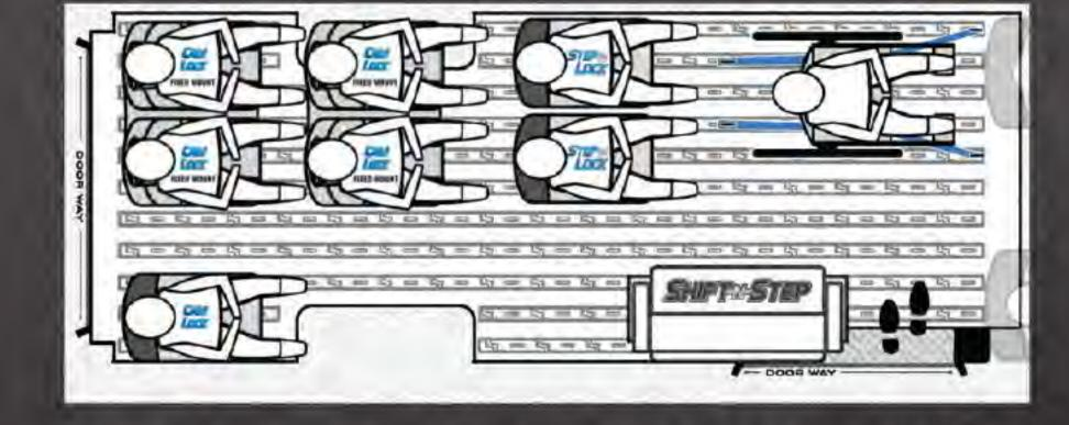
Example Floorplan of an AbiliTrax 170 Class Shift N Step
